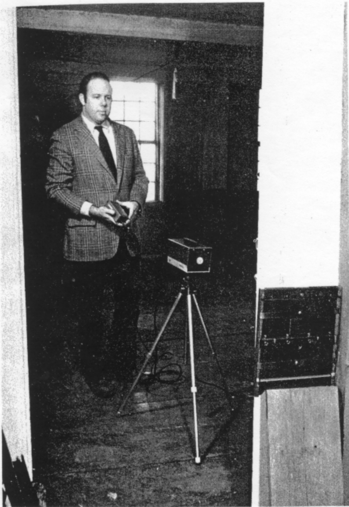
Fig. 1 Author David Hart with portable X-ray generator (on tripod) and film holder (seen on near side of doorway).
